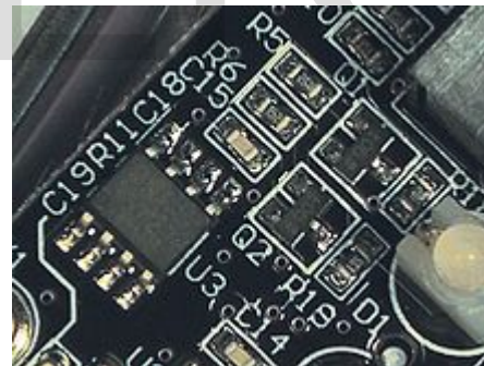
Surface mount components, including resistors, transistors and an integrated circuit
